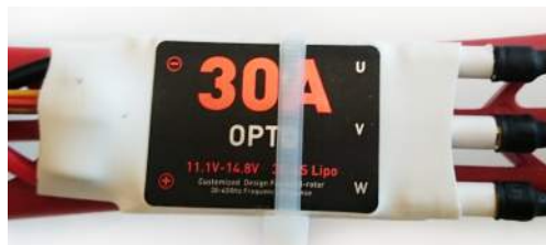
Figure 5: Picture of an Electronic Speed Controller (ESC) that controls the speed of the motors.
