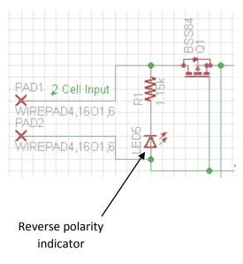
A mechanism needs to be implemented such that if the battery is plugged in incorrectly, the system will automatically prevent backwards circuit flow, eliminating risk to safety. For this purpose, a p-channel MOSFET was chosen. If the battery is plugged in backwards, current will flow through the MOSFET in a forward biased manner, causing the LED to light, thus indicating a reverse polarity situation. A shunt resistor of 1.15 k $\Omega$  was chosen.
