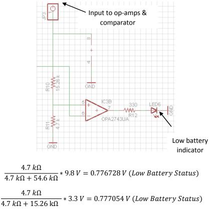
If the voltage read by the ADC reaches 0.777 V, this means the battery is low, and the comparator will trigger, thus lighting the low voltage LED.
