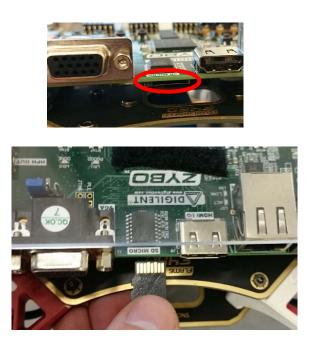
18. Once the card is in, simply turn ON the board and you should see the green Done LED come on (indicating the FPGA was configured successfully) and the program will start executing a few milliseconds after
